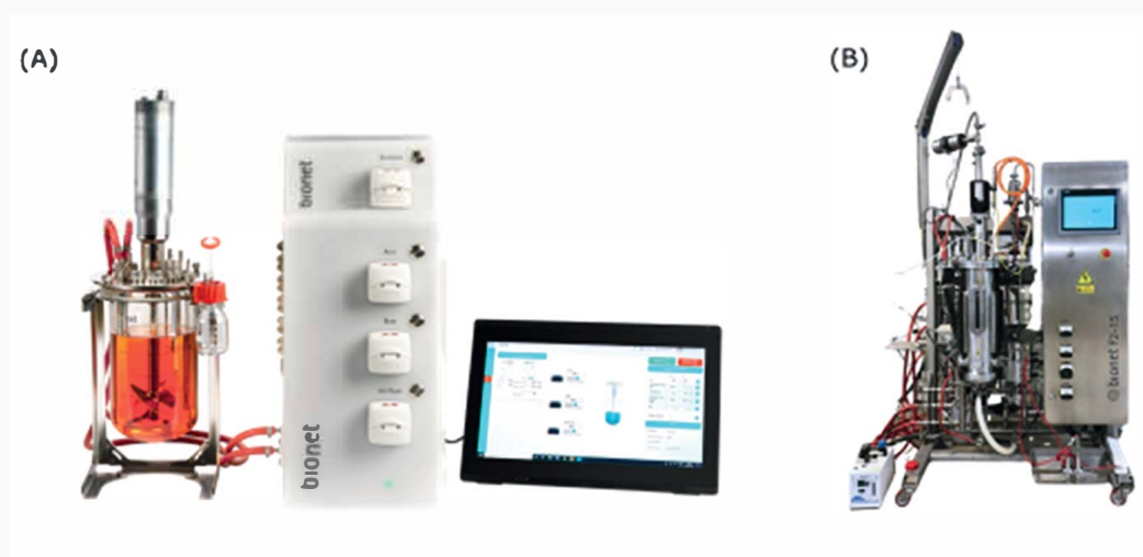
Figure 4. Bioreactors used for experiments: (A) laboratory-scale bioreactor Bionet FO-2CC and (B) pilot-scale bioreactor Bionet F2-15MB.
