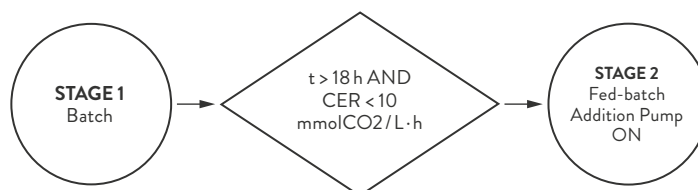
Fig. 4: Example of the scheme of transition configuration between stages using CER to activate an addition pump.
