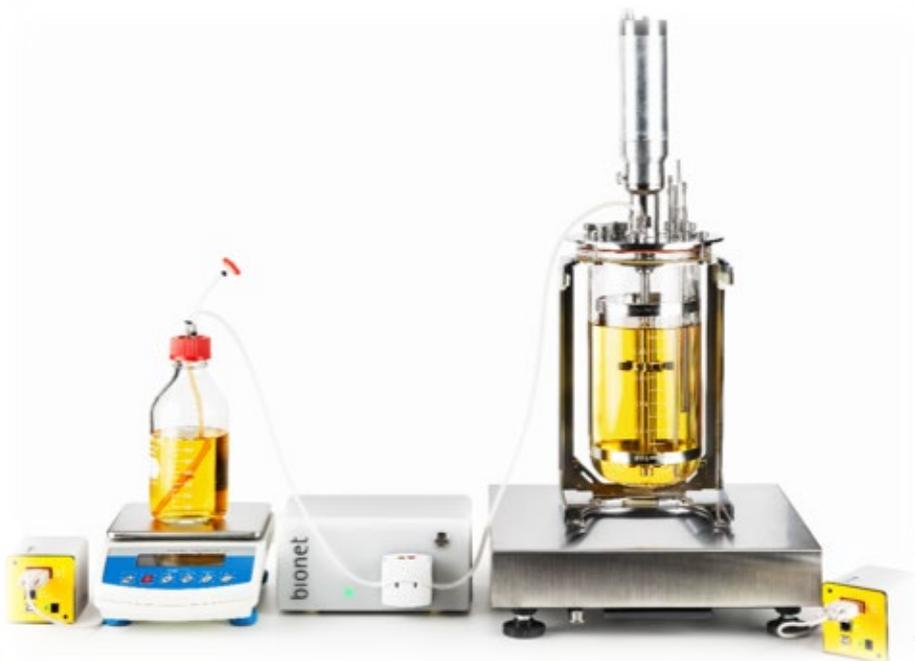
**Fig. 1:** Set-up of an addition weight control for a fed-batch by a Bionet system, where the bottle of the substrate is placed on a scale for precise addition control and weight data visualization and registration and where the bioreactor is also placed on a scale for bioreactor weight data visualization and registration. Both will be recognized by the software via the bScale modules also shown in the picture.
