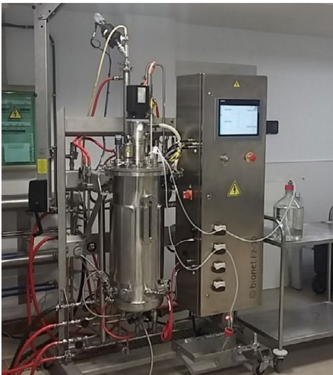
Fig.2: Bionet F2-30A stainless steel Bioreactor used for the scale-up, autonomous configuration (no steam installation needed for sterilization). Available in 15 and 30L working volume models, and autonomous or non-autonomous configurations for sterilization.
