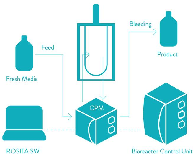
**Figure 1.** Continuous fermentation process at lab scale by using a BIONET FO-BABY bioreactor with a Continuous Process Module (CPM).
