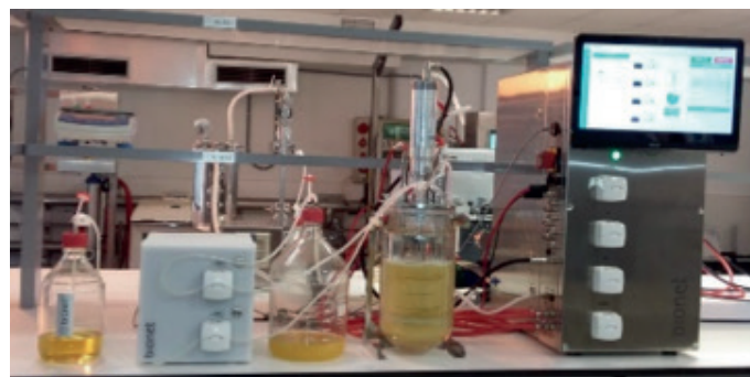
Fig.2. Set-up of the semi-continuous system for the fermentation of P. pastoris in Bionet F1 MB Bioreactor model accompanied by the Continuous Process Module (CPM).
